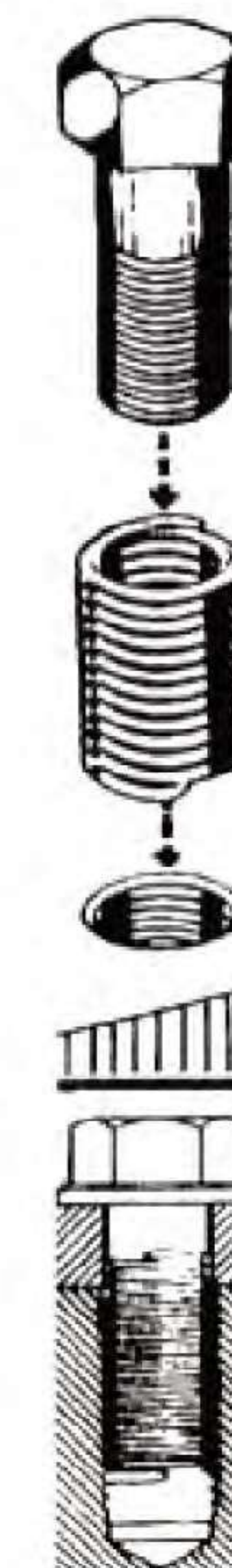
Fix the screw thread insert with the installation tool
